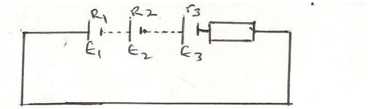
$$\begin{aligned} \text{Total internal resistance, } r_T &= r_1 + r_2 + r_3 \\ &= 2 + 2 + 2 \\ \therefore r_T &= 6\Omega \end{aligned}$$
