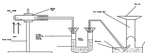
1. Heat potassium trioxochlorate V and manganese iv oxide in the ratio 4:1 by mass in a hard test tube fitted with a delivery tube.
